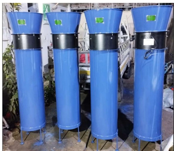
Onion Storage Blower
